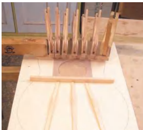
STEP 10. Clamping the harmonic bars
